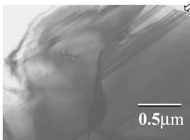
Fig. 2 Low-magnification bright field TEM image of the \text{Li}_2\text{MnO}_3 sample showing micrometer-size grains with platelet-like defects (see arrow) localized in areas of some hundreds of nanometers
